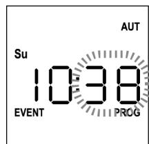
7. Set the minutes using the **UP** and **DOWN** keys and press the **MENU** key to confirm.
