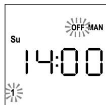
4. Using the **UP** and **DOWN** keys, select the **ON** (active) or **OFF** (off) state of the channel, press **MENU** to confirm and proceed to the next channel.
