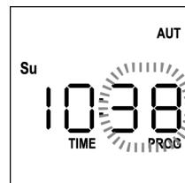
7. Set the minutes using the **UP** and **DOWN** keys and press the **MENU** key to confirm.
