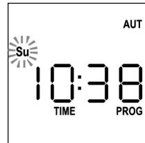
5. Set the correct day using the **UP** and **DOWN** keys and press the **MENU** key to confirm.
