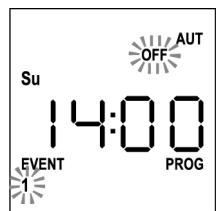
8. Set the channels which must transmit for this event: using the **UP** and **DOWN** keys, select the **ON** (active) or **OFF** (off) state of the channel, press **MENU** to confirm and proceed to set the next channel.
