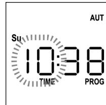
6. Set the time using the **UP** and **DOWN** keys and press the **MENU** key to confirm.
