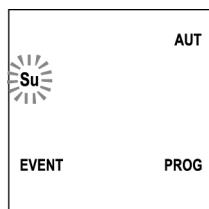
4. Select the day on which you want to set up the event by using the **UP / DOWN** keys and press **MENU** to confirm.
