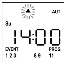
**13.** Select the desired event using the **UP** and **DOWN** keys and press **MENU** to confirm and proceed.
