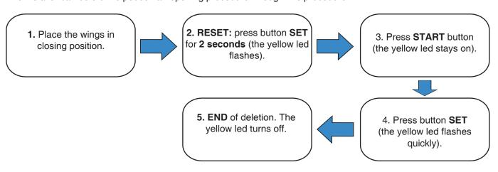
After the deletion, it will be possible to activate the pedestrian opening only by wire, and the size of the opening will be total on the wing opened by MOT1 (terminals 24,25)
