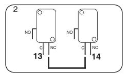
① If there is more than one stop contact, they must be connected in series (see picture 2).
